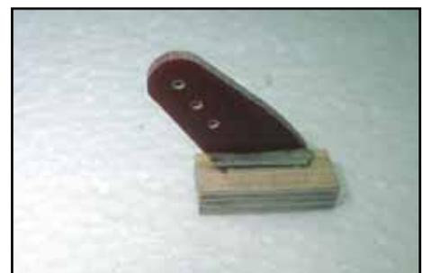
and connect the speedbrake to the servo output arm, which should be of the heavy-duty type. In the 'closed' position the servo arm should angle forwards at about 45 - 50 degrees.
