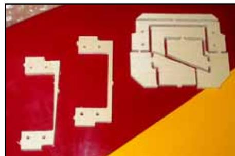
(above) Shows the tapered and parallel top servo mounting rails.
