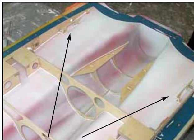
(above) Milled plywood rudder servo mounts are installed during the mould joining process.
