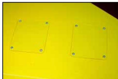
Trial fit the servos into the wing with the servo hatches and adjust the position so that the servo arms line up exactly with the phenolic control horns. Rough up the inner surface of the hatches carefully with 80 grit, and glue the servo mounts on with a drop of CA. Check position, and when satisfied glue them on securely with a good fillet of epoxy. These are important joints so make sure to prepare the surfaces well before gluing together.
